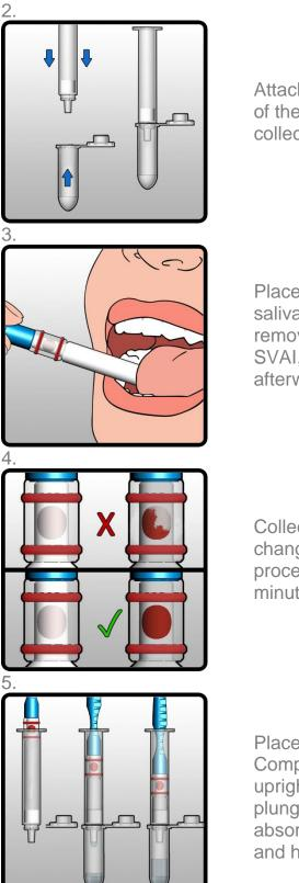
Attach the Eppendorf tube provided to the base of the Compression Tube firmly. Sample collection may now begin.
