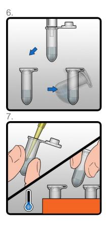
Gently remove the Eppendorf Tube from the end of the Compression Tube. Add preservative (not provided), if required, and close the lid tightly. Invert the tube 2-3 times.
